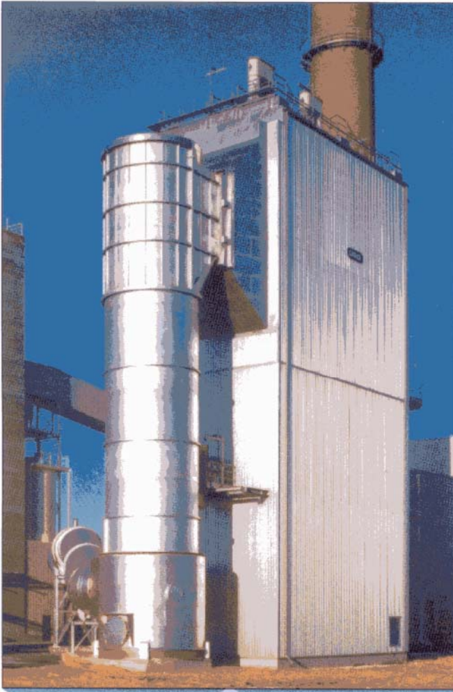
Reactor with Soda/H 2 O-Additiv and Electrostatic Precipitator
